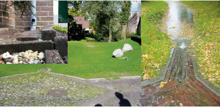
retaining precipitation by 'wadi' system (groundwater recharge)
